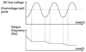
Figure 6-26 Diagram of the overvoltage stall protection function
