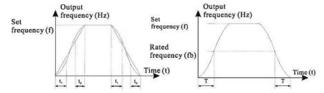
Figure 6-2 S-curve acceleration/deceleration/Agure 6-3 S-curve acceleration/deceleration B
