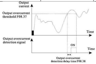
Figure 6-23 Output overcurrent detection
