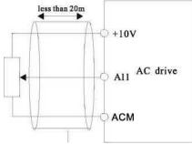
Figure 3-5 Schematic diagram of analog input terminal wiring
