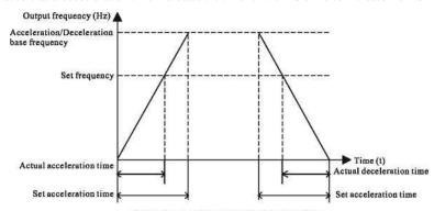
Figure 6-1 Acceleration/Deceleration time
