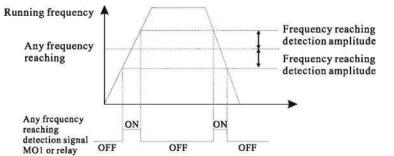
Figure 6-21 Any frequency reaching detection
