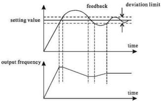
Figure 6-29 relation between deviation limit and output frequency
