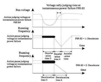
Figure 6-25 AC drive action diagram upon instantaneous power failure F09.02 = 2, upon instantaneous power failure or sudden voltage dip, the AC drive decelerates to stop.
