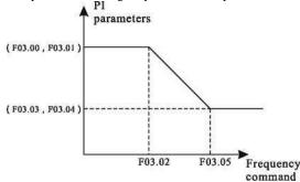
The speed dynamic response characteristics in vector control can be adjusted by setting the proportional gain and integral time of the speed regulator.
