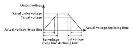
Figure 6-8 Voltage of V/F separation
