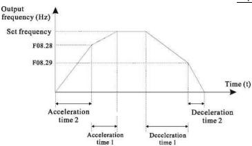
Figure 6-20 Acceleration/deceleration time switchover
