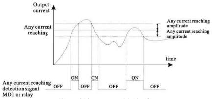
Figure 6-24 Any current reaching detection
