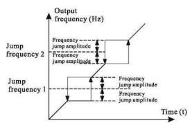
Figure 6-15 Principle of thejump frequencies andjump amplitude
