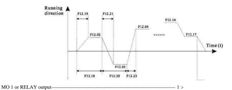
250ms pulses Figure 6-34 Simple PLC when used as frequency source
