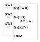
Figure 6-11 Setting of 3-wire control 1
