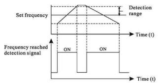
Figure 6-18 Detection range of frequency reached
