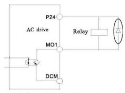
Figure 3-7 Wiring diagram of digital output terminal
